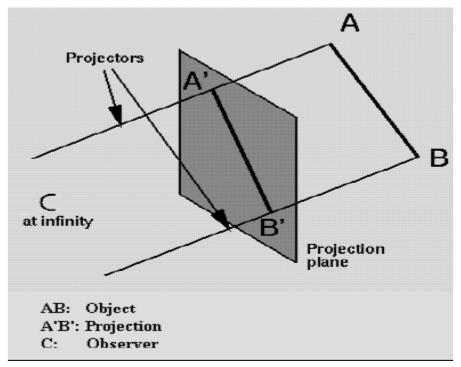
Parallel Projection is a type of projection where the line of sight or projectors are parallel and are perpendicular to the picture planes. It is subdivided into the following three categories: Orthographic, Oblique and Axonometric Projections.
