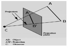
Perspective projections are drawings which attempt to replicate what the human eye actually sees when it views an object. There are three types of perspective projections: One-point, Two-point and Three-point Projections.
